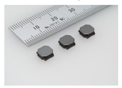
Taiyo Yuden Co., Ltd. has added a new product with height 2.8mm, the NR6028 (6.0x6.0x2.8mm, height is maximum value), to its wire wound power inductor NR60 series lineup used as choke coils in LCD TVs and plasma TVs. This product improves the rated current by about 36% over previous Taiyo Yuden products (inductance 10μH).
